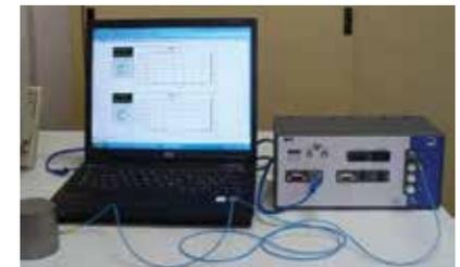
Fig. 7 Fiber optic sensors interrogation system
