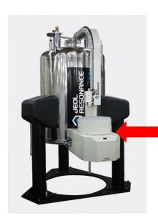
A cooled autosampler for 30 tubes will be provisionally provided on approval
