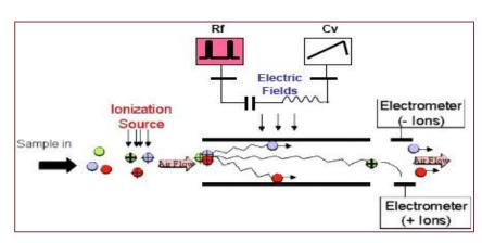
DMS identifies and detects chemicals based on a chemical species ion mobility, which depends of ion dimension (geometry) and charge, in low and high electric fields. The DMS device can be used as a filter (improved selectivity) or in scan mode (improved characterization)
