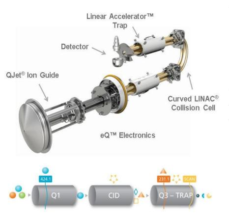
A QTRAP is based on the conventional ion path of a QqQ mass spectrometer. However, the third quadrupole (Q3) can also be operated as a **Linear Ion Trap (LIT)**. The dual functionality of Q3 provides to the system complete functionality as a QqQ mass spectrometer, with great sensitivity for quantitative measurements, but with additional powerful scan functions.
