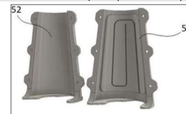
Fig. 3 External mold covers for the silicone skin.
