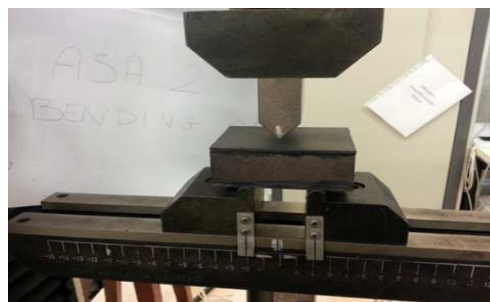
Fig. 3 Bending on the structure / Bending on sandwich.
