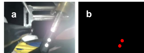
Fig. 3 Software implemented: a) acquisition of the video of the movement; b) elaboration of the markers placed on the device.
