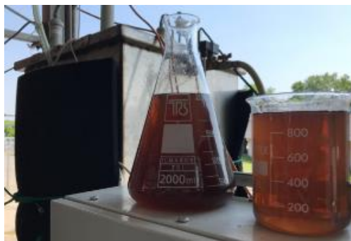
Fig. 6 Feedstock fermented after the second filtration step, used in the PHA production phase.
