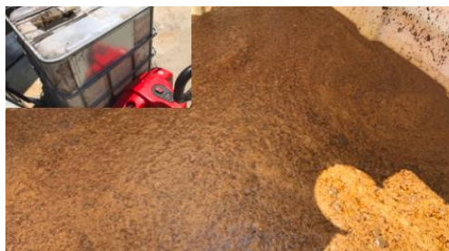
Fig. 3 Pre-treated Feedstock (on entry to the acidogenic fermenter).
