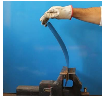
Fig. 5 Prototype: first clamped stable configuration at fixed load, point C1 on Fig. 2.
