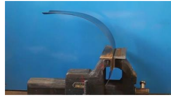
Fig. 4 Prototype: clamped stable shape without applied loads, point O on Fig. 2
