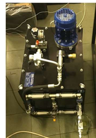
Fig. 6 G.L.E.S. prototype (oleo dynamic system and oil pump).
