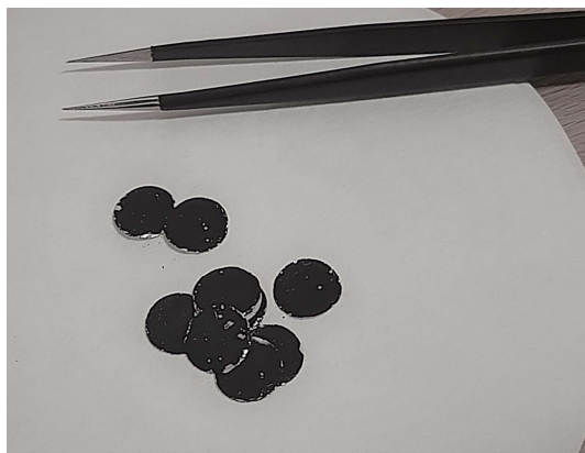
Fig. 4 composite electrodes constituted by lithium rich layered oxides.
