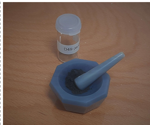
Fig. 1 Lithium-rich transition metal mixed oxide.
