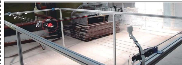
Fig. 2 Sketch of a prototype for a cable robot with 2D workspace.
