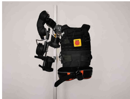
Fig 1. SIDE exoskeleton in front view on his support.
