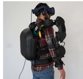
Fig 4. Lateral view of the subject wearing SIDE. You can see the backpack containing the control electronics.
