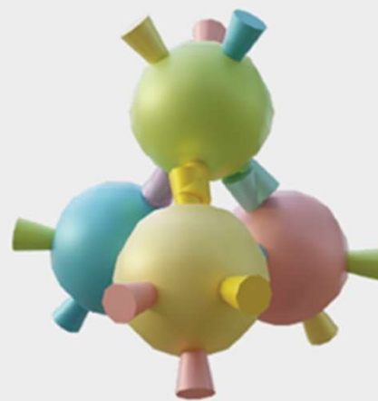
Fig.1 Patchy particle model for the building blocks, comprising 4 species and 24 individual bonds..
