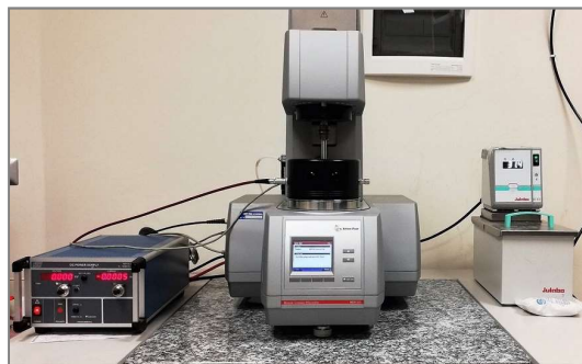
Fig. 1 Measurement setup, including, from left to right, the DC voltage supply, the rotational rheometer and the thermostat required to cool down the Peltier cell integrated underneath the lower plate.
