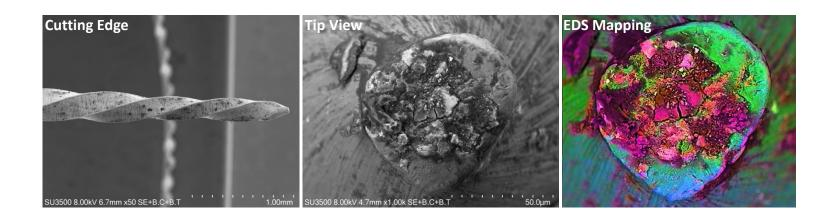
Endodontic rotary alloy instruments for root canal configuration.
