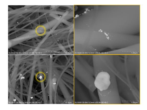
Sensing properties depend on the morphology, crystallinity and chemical composition of the functionalized Gold Nanoparticles deposited onto quartz fibers able to reveal very low concentrations of gaseous mercury
